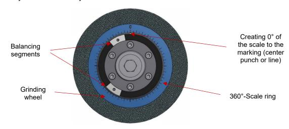
If no flange with balancing segments available, please ask for MPM balancing rings.
